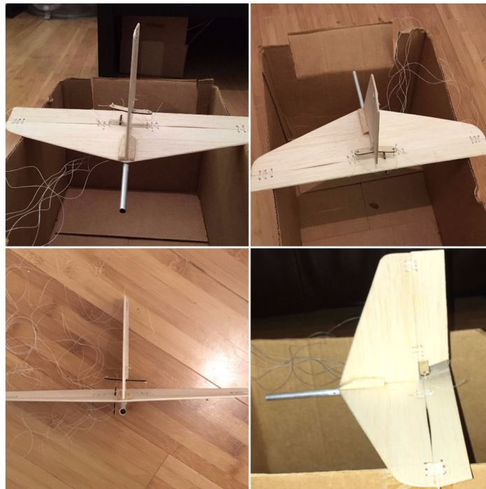
Figure 12 :Top, side and front view of tail
